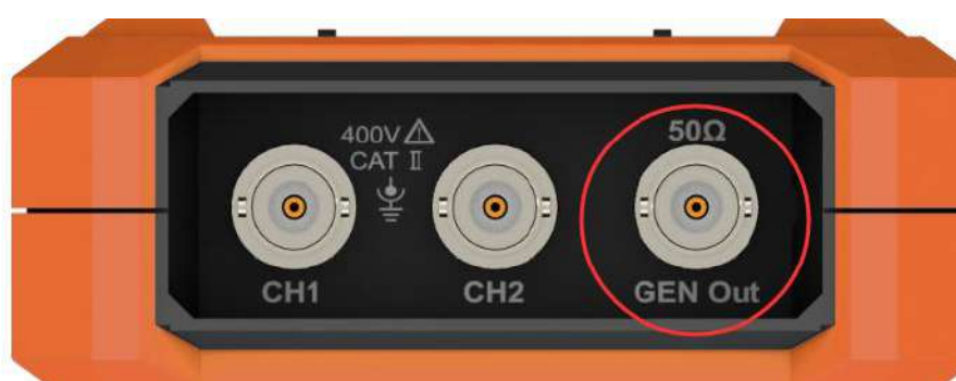
Figure 5- 1: Generator Output Ports
