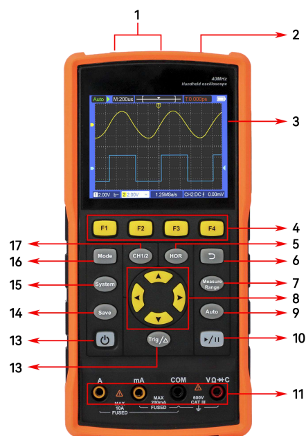
Figure 4: Front Panel of the Oscilloscope
