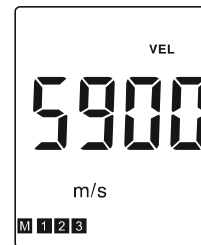
Last applied sound velocity & registered unit
