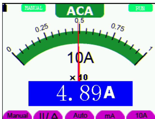
Figure 30: AC Current Measurement for 10A
