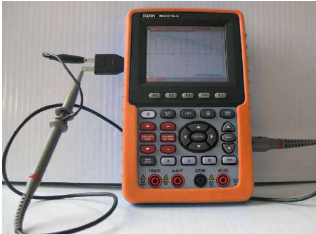
Fig.3. The connection of Square-wave test signal
