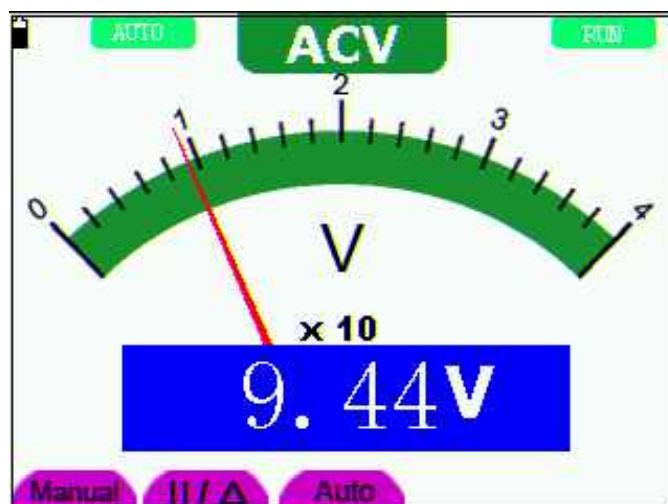
Figure 23: AC Voltage Measurement
