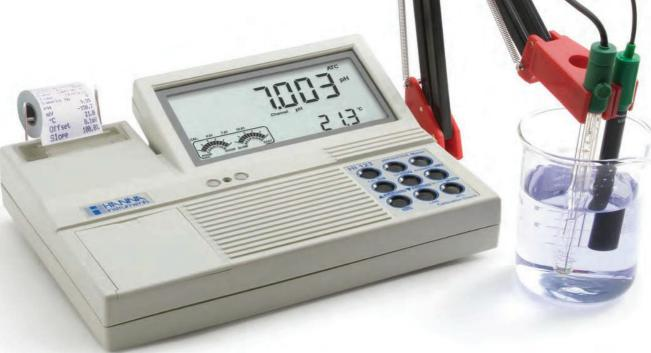
HI 122 and HI 123 are benchtop instruments featuring a built-in printer, Calibration Check $^{\text{TM}}$ , electrode response time and condition monitoring, and enhanced diagnostic messages during calibration. HI 123 also incorporates dual inputs to measure both pH and ISE simultaneously.
