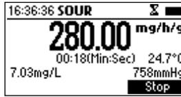
At the end of the analysis the meter will display the computed *SOUR* value, the duration of the measurement, and the pressure and temperature values. Press **Log** to record a record of this analysis.
