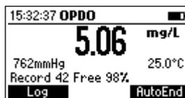
The meter will display for a couple of seconds the record number and the amount of free space (in %). If the maximum number of stored measurements is achieved, the “**Log space is full**” message will be displayed for a few seconds when **LOG** key is pressed.
