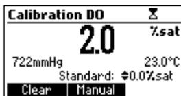
The *DO* calibration screen will be displayed and the standard 0% saturation (or 0 mg/L, depending on the currently selected measuring unit), will be automatically selected.
