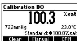
**Two points automatic calibration at 0% saturation (0 mg/L) and 100% saturation (8.26 mg/L)**
