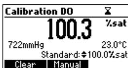
The *DO* calibration screen will be displayed and the standard 100% saturation (or 8.26 mg/L, depending on the currently selected measuring unit), will be automatically displayed.
