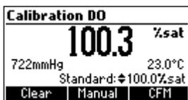
When the reading is stable within the acceptable range, the *CFM* functional key is displayed.
