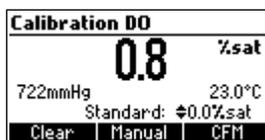
Press **ESC** to leave calibration or continue for a two point calibration.
