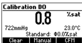
Press **CFM** to confirm the calibration point.
