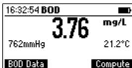
Press **BOD Data**. The following screen will open. Place the probe into the *BOD* sample and allow the measurement to stabilize. The sample should be well mixed. Follow all standard operating procedures.
