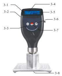
3-1 Unit N3-6 Zero Key3-2 RS232C Interface3-7 Power Key3-3 Calibration Key3-8 Indenter3-4 Display3-5 Measurement Value
