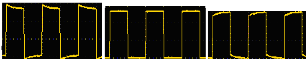
Figure 3-6 Displayed Waveforms of the Probe Compensation
