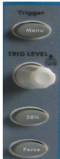
Figure 4-14 Trigger Control Zone
