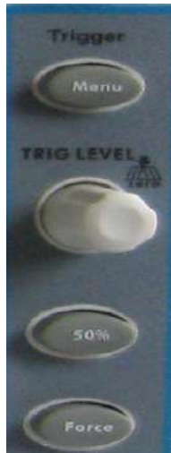
Figure 4-14 Trigger Control Zone
