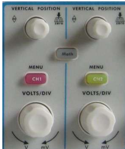
Figure 4-12 Vertical Control Zone
