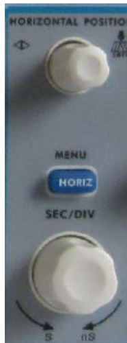
Figure 4-13 Horizontal Control Zone
