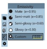
As shown in the figure, press "0/MENU" key to enter the main menu and select "  $\mathcal{E}$  "(emissivity) option and press "  $\blacktriangleright$  " key to enter the emissivity list.
