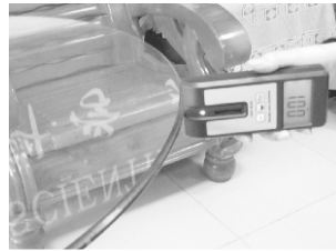
figure 1: Correct method of placing Model 1000 on glass.
