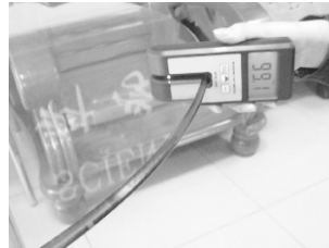
figure 2: Model 1000 correctly seated on glass to be measured.
