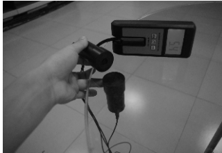
figure 1: Correct method of placing Model 1100 on glass.
