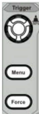
Figure 3-12 Trigger Control Zone
